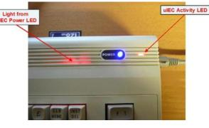
Figure 2 - Blue Power LED and activity LED from uIEC
