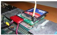
Desoldered original power LED and substituted 2-pin header Connect a normal PC "Turbo" (or HDD) LED ! Hardwired into IEC bus on underside of motherboard
