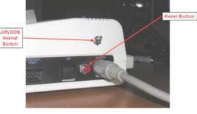
Figure 3 - JiffyDOS switch and reset button
