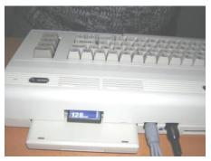
Figure 4 - Cutout above cartridge slot for Compact Flash card
